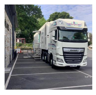
The area in which our mobile scanner is to be sited should always be clear for access so that the unit can be positioned correctly. The surrounding area must also be a sound surface to provide good access to the trailer.
